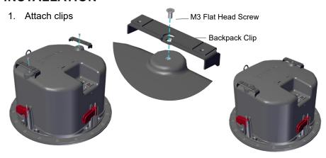
2. Fully slide unit into clips
