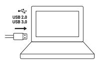
**4.** When a USB device is connected, the speakerphone will automatically power on.
